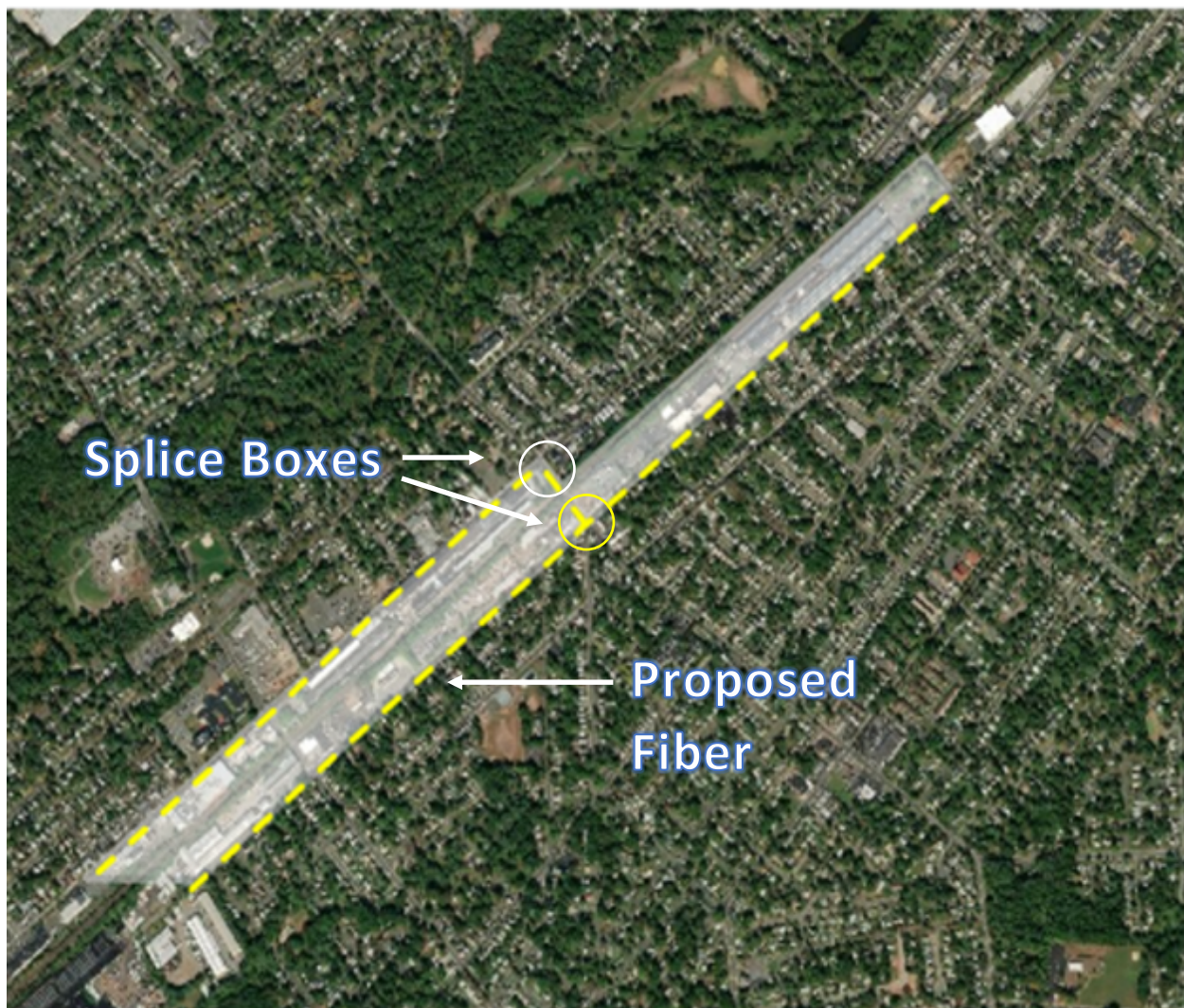
Figure 18: Proposed Fiber Routes with Splice Boxes
